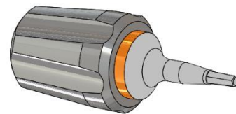
FIG.4 : Screwdriver Adapter Mounted
