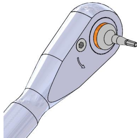
FIG.8: The screwdriver in the mounted position
